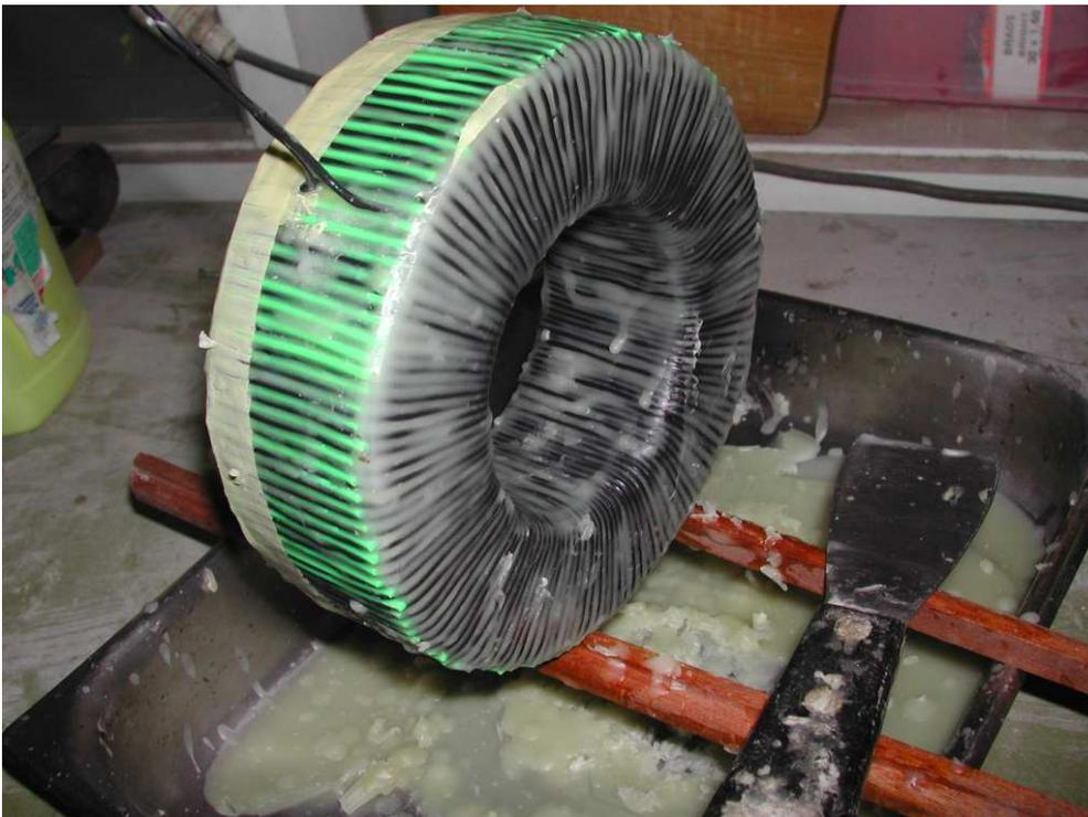
*When finished, tape with glass tape and PE tape being careful not to damage the flying leads.*
