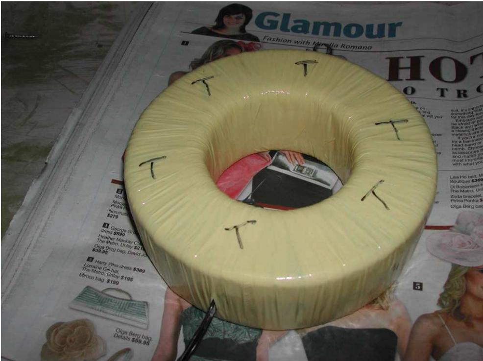
13. Now it's time for the secondaries. I made a layout drawing in Autocad and PDF showing the  $120^\circ$  separated "centre" lines of the primary coils and also the angle that the coils that I wound took up. Print this out, lay it on the top face of the toroid with the centre point of one winding centred on the secondary flying leads and mark the end points of the windings.
