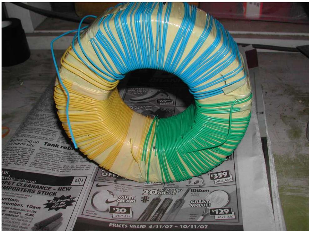
15. Then check locations, tape firmly in place and fit spacers.
