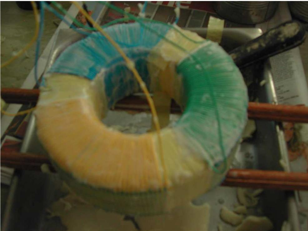
17. Final tape. If you want a low voltage sensor loop wind between two primaries before taping.
