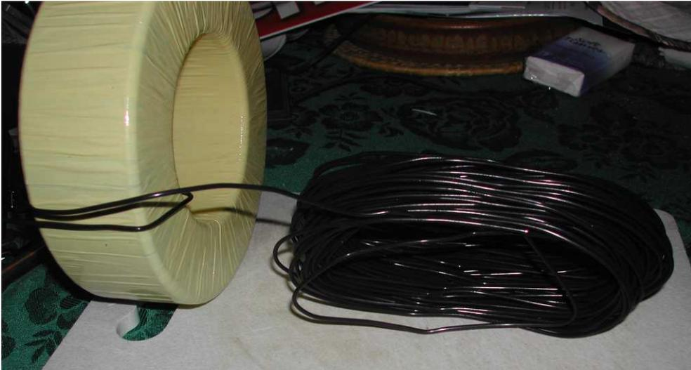
3. Mark the top face of the toroid with a biro or felt marker and also the start of the larger secondary winding wire with some doubled PE tape and a marker.
