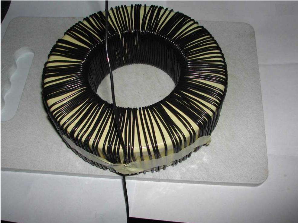
7. Count the windings (that pass through the hole) and record it somewhere- I got 129 and marked this on tape on one end of the winding itself. I counted by making marks on the yellow tape on the outside of the toroid every 5 turns with a black felt pen. It did make it a little harder to judge the spacing later and I wish I hadn't....
