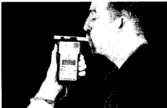
Figure 2.5 Fuel cell-based breathalyser as used by police forces in the USA. (Reproduced by kind permission of Lion Laboratories Ltd.)
