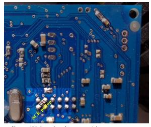
SCK pullup = 4k7 diagonally on ISP header, bottom side
